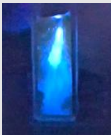
Chemiluminescence of luminol injected into a cuvette with a catalyst
