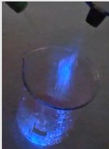
Tested in two impinging sprays to visualize their interaction zone
